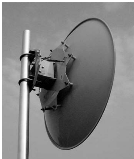
The MPR's compact and light weight spun aluminum reflector provides maximum parabola accuracy for more consistent and reliable antenna performance. Its robust mounting structure prevents bending and oscillation that can cause signal degradation.
